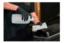
Note: No other cleaner (surface cleaner, etc.) may be used for the final surface pre-cleaning, as this can attack the adhesive on the CYS TPU and have a negative effect.
