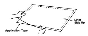
Squeegee the graphic from the liner side to adhere the application tape. Work from the center out. See FIGURE 4.
