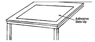
2. Align the graphic face-down on the application tape adhesive. See FIGURE 3.
